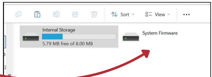
6. The controller will automatically update the firmware and reboot. (Note: The controller will default to factory settings. You will need to enter configuration and set-points again.)
