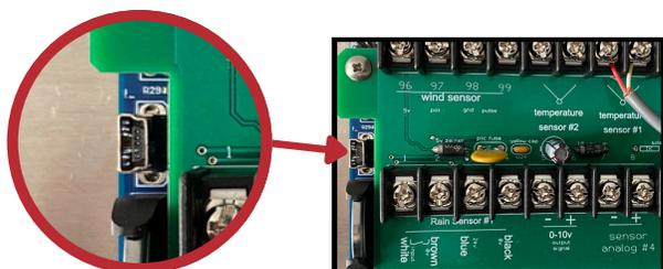
**Note: Data cable is connected to the same port that was used for dropping code.**
