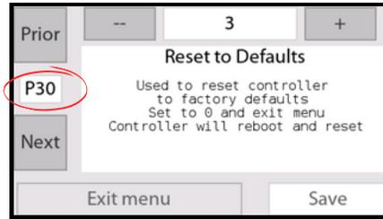
2. Set P30 to “0” using the plus (+) or minus (-) button and then press Save. And then exit menu. The controller will reboot.
