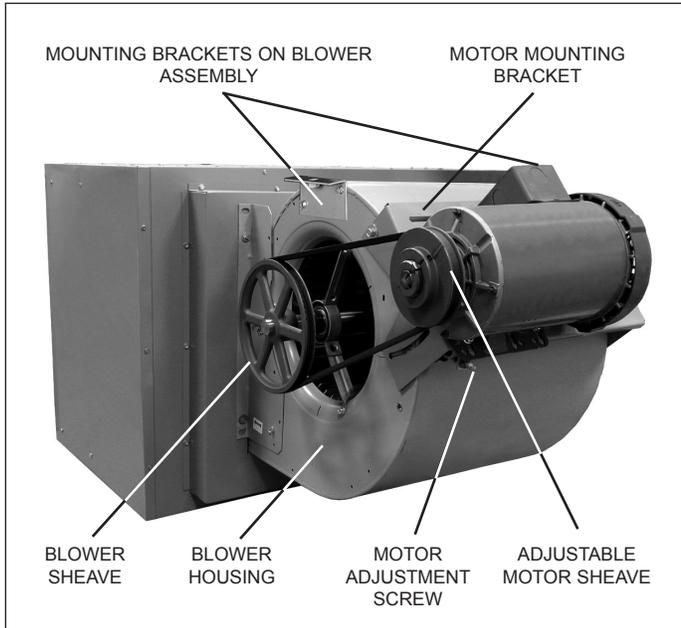
3. Adjust motor adjusting screw for a belt deflection of approximately 3/4" with 5 pounds of force applied midway between the sheaves (refer to Figure 19.3). Since the belt tension will decrease dramatically after an initial run-in period, it is necessary to periodically re-check the tension. Excessive tension will cause bearing wear and noise.
