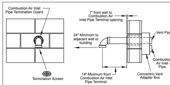
D3. Once the kit contents have been verified as correct for the direction of venting, the concentric vent adapter box is to be installed. Determine the location of the box. Be sure to maintain all dimensions as listed in these instructions.
