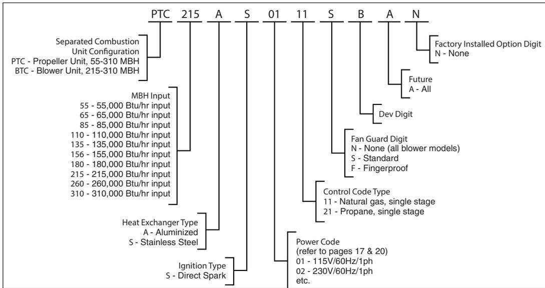
**Figure 31.2 - Serial Number Designations** (Remove access cover to locate)
