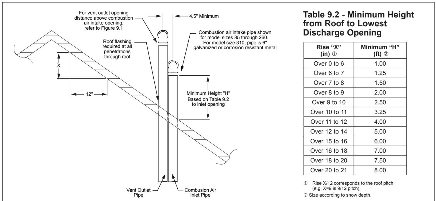
Table 9.2 - Minimum Height from Roof to Lowest Discharge Opening
