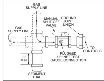
① Manual shut-off valve is in the "OFF" position when handle is perpendicular
