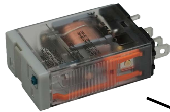
490-CR1P24DC Cube Relay, 24 VDC coil voltage, SPDT, 15A contact rating, 5-pin, LED Indicator
