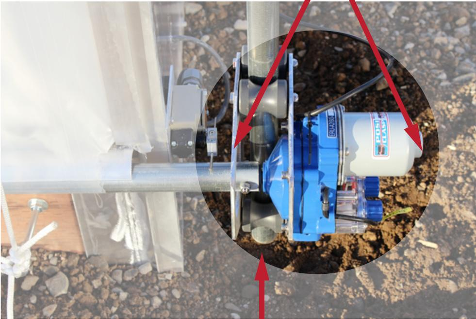
2-3" between the edge of the greenhouse and the guidewheel unless you are using roll lock. When using roll lock you need an external limit switch to control the downward movement of the motor.
