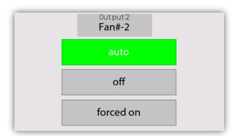
Select the relay status you want. In Auto it will operate automatically. Selecting Off or Forced allow you to avoid the control system. To exit press the blank space on the sides.
