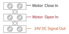
All connections to the environmental control must be made to dry contacts!
