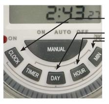
To set the day or time press and hold the "Clock" button. Then select the Day, Hour or Minute button to make the necessary changes.
