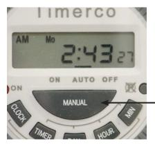
When pressed the manual override button cycles between the On, Auto, and Off functions of the timer. In order for the timer to open and close your curtain during the preset time periods it must remain in Auto.
