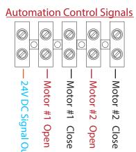
All connections to the environmental control must be made to dry contacts!
